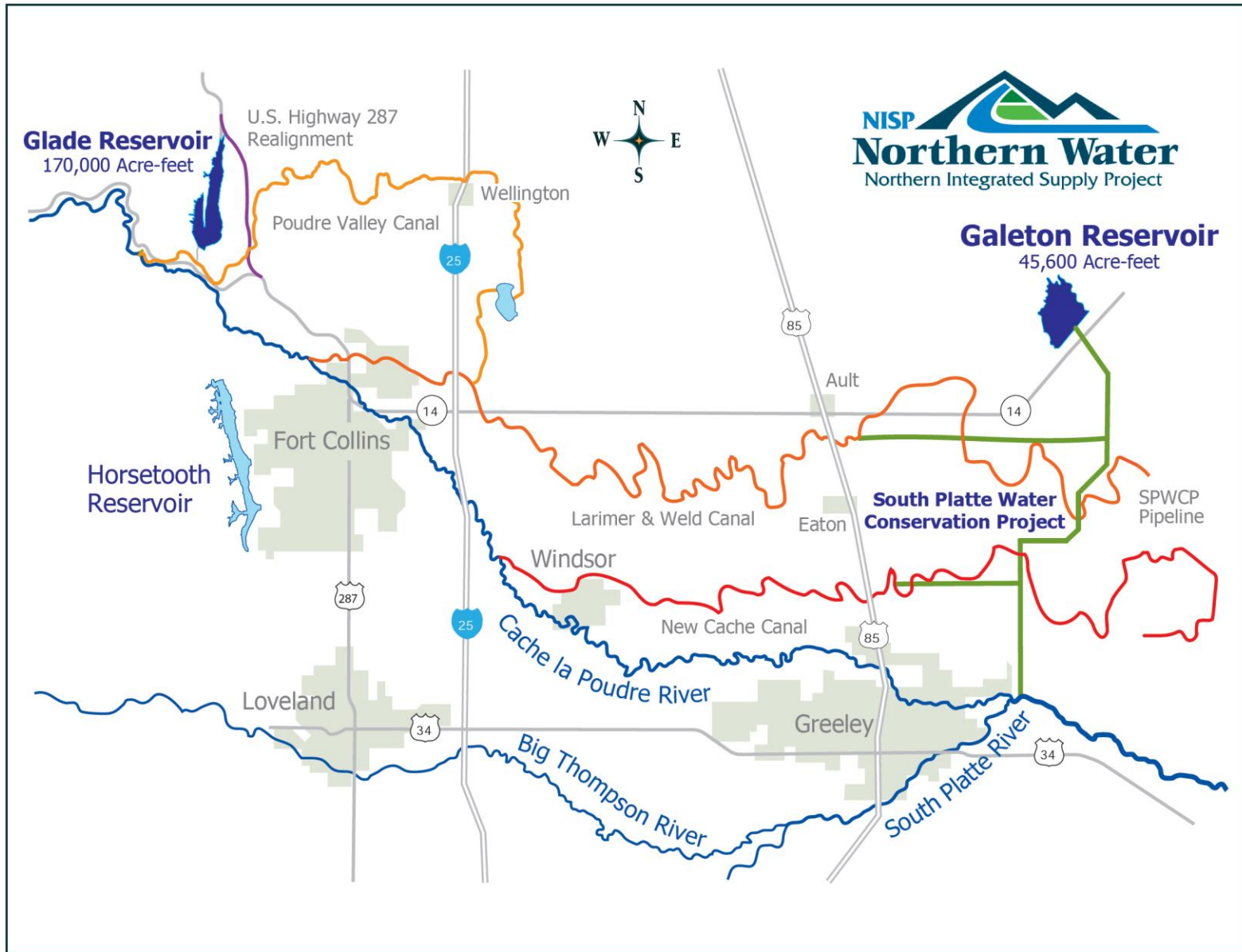
Figure 1. NISP Infrastructure and Features
