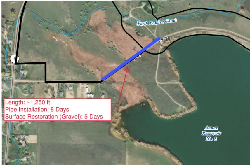
WORK SITE DETAIL
