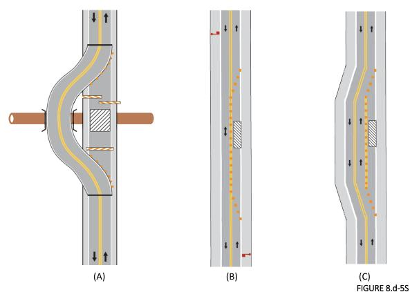
(A) Road Closure with Diversion, (B) Partial Road Closure with Flaggers, (C) Road Closure with Diversion
