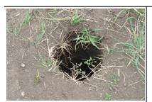
Percolation tests are not required if two soil test pits are evaluated by the engineer or system designer. If percolation tests are performed they must follow the guidelines in the regulations. Two test pits must be dug regardless of whether percolation testing is performed or not.
