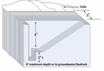
As of June 4, 2018 all applications for a new on-site wastewater treatment system must include an inspection of two test pits as part of the site and soil evaluation. All site and soil evaluations must be made by or under the supervision of a professional engineer.
