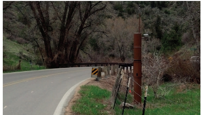
Several rain gages were installed to provide information on flooding following the High Park fire.
