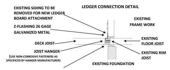
1/2" LAG BOLTS OR LAG SCREWS AT 16" ON CENTER OR **LEDGERLOKS** PER **MANUFACTURER'S** SPECIFICATIONS (WHICH MUST FULLY PENETRATE THROUGH THE RIM BOARD). REFER TO ATTACHED TABLE FOR QUANTITY.
