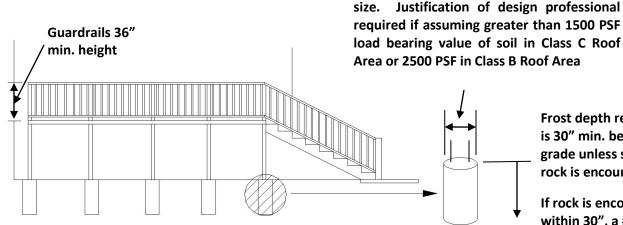
Frost depth required is 30" min. below grade unless solid rock is encountered.
