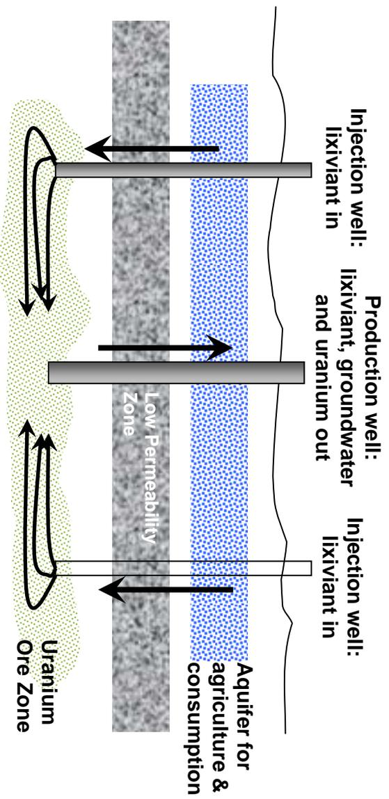
Figure 1: Schematic of ISL operations
