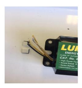
5. Bring the ballast and fluorescent bulbs to the HHW facility. Throw away the plastic cover, recycle the metal exterior at a scrap metal recycler.
